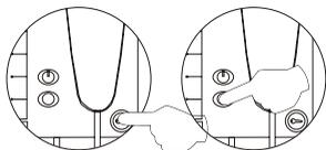
Turn off the monitor to be set, by pressing the door opener button during 1 second.
