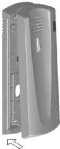
Pass the installation wires through the corresponding hole and connect them as shown on the installation diagrams. Close the telephone as shown on the picture. Once the telephone is closed, connect the handset using the telephone cord and put it on the cradle.
