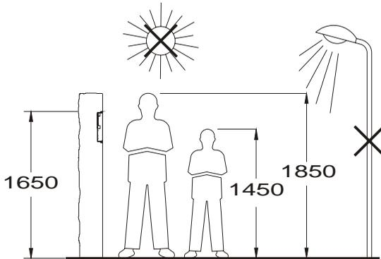
The upper part of the door panel should be placed at 1,65m. height roughly. The hole dimensions will depend on the number of door panel modules (see page 108).:
