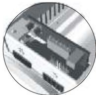
*Platea PLUS:* Locate the CN4 connector, that's placed in the monitor base. Remove the existing jumper and plug the EL562 module.
