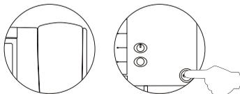
To set up the monitor as the main one, hang the handset up.
