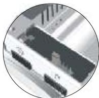
The end of line jumper is placed on the CN4 connector (CN2 on Platea UNO), that can be located on the monitor base.
