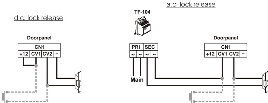
The lock release can be activated at any moment by using an external push button, that must be connected between 'CV1' and 'CV2' terminals, as shown in the diagram. This function will allow to exit from the building being not necessary the use of a key.
