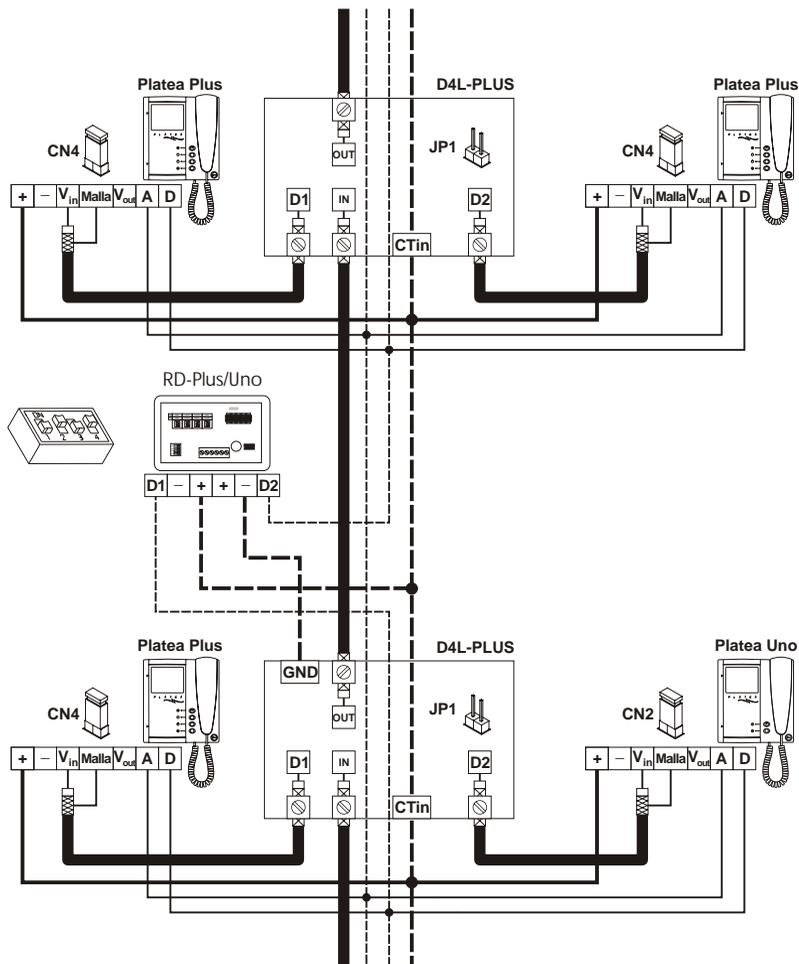
An easy way to check that the system is working properly is to disconnect the wiring from the door panel and to check the monitor directly connected to the door panel terminal connector.
