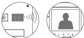
The doorpanel will produce tones to indicate that the device is ready to be set up.
