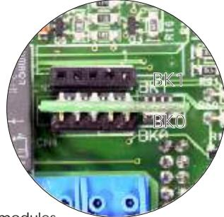
**IMPORTANT:** in case of doorpanels with two memory modules, don't change their bank position once they have been recorded. BK0 bank module must always have a memory module plugged in.
