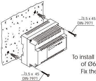
The power supply must be installed in a dry and protected place. It's recommended to protect the power supply by using a thermo-magnetic circuit breaker and to use a ground connection.
