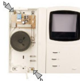
Remove screws b, in order to take off the bottom part of the handset.
