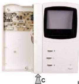
Unscrew screw c and remove middle cover.
