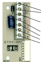
Connect terminals '0' and '8V' to optional (separate) 8VAC power if you wish to use the built-in LED light(s)
