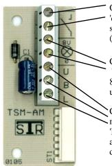
Optional set of momentary 'dry' contacts for push-button on speaker/microphone module (with lamp symbol)
