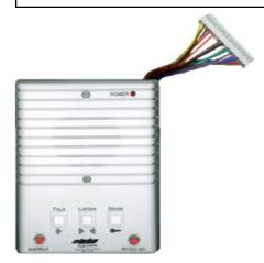
The CP001B tester is used to test PK543 and PK543A amplifiers for proper operation of the four basic functions (Talk Down, Talk up, Ring Up, and AC Door release).
