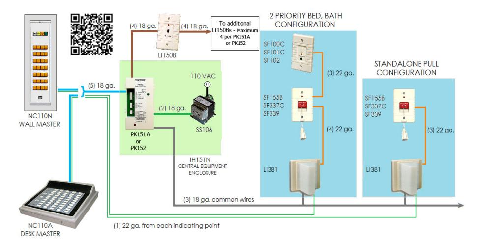
This diagram represents a typical basic system. For more specific details and variations, please refer to the NC110A - NC110N Installation & Operation Manual IL381.
