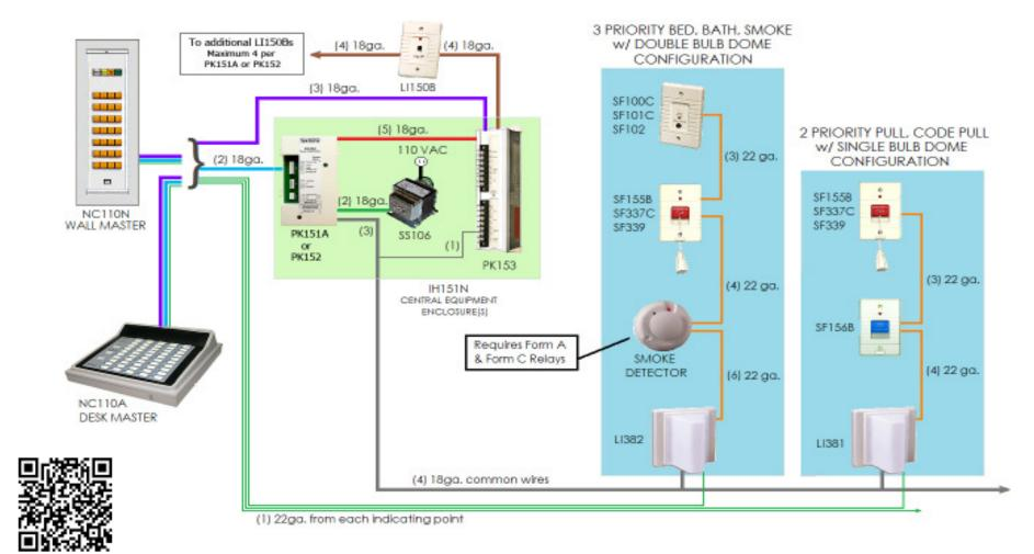
This diagram represents a typical basic system. For more specific details and variations, please refer to the NC110A - NC110N Installation & Operation Manual IL381.
