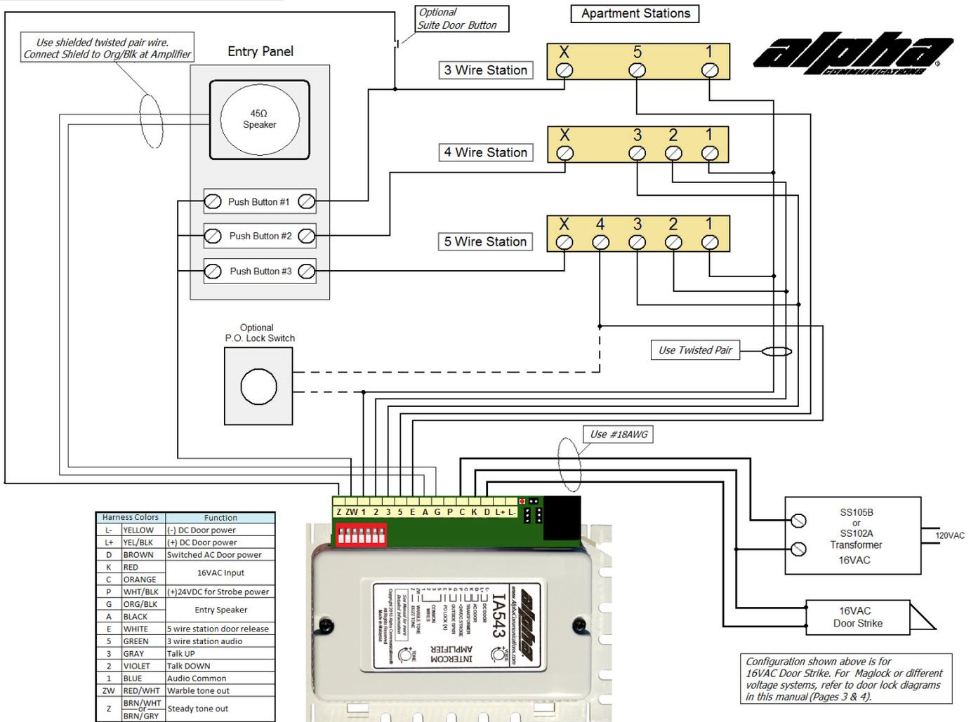
The IA543 amplifier has two serviceable adjustments for Voice Volume and Tone Volume located through two access holes on the front cover. Use a small screwdriver and do not use excessive force. Carefully turn clockwise to increase the volume. High volume setting may result in feedback oscillation.
