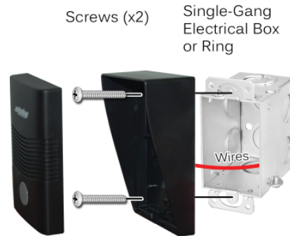
Figure 2: OR222 Mounting Diagram
