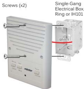
Figure 3: Typical Wiring for one Indoor Master Station
