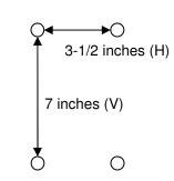
• Wall-Mount Brackets at Left & Right edges of the sign (brackets rotated 90-degrees from above):
