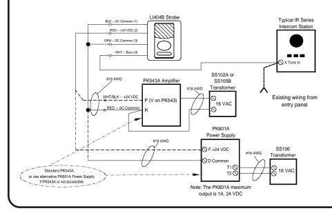
per apartment are used, a PK601A Power Supply must be used in conjunction with the PK543A Amplifier to supply power to the strobes.
