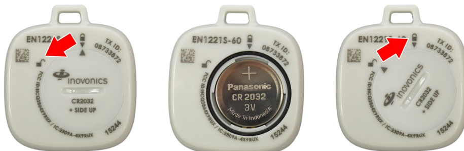
Figure 64: SF503ES and SF504ES Battery Replacement
