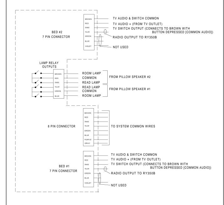
NOTE: PM321B lamp does not include top 7-pin module.
