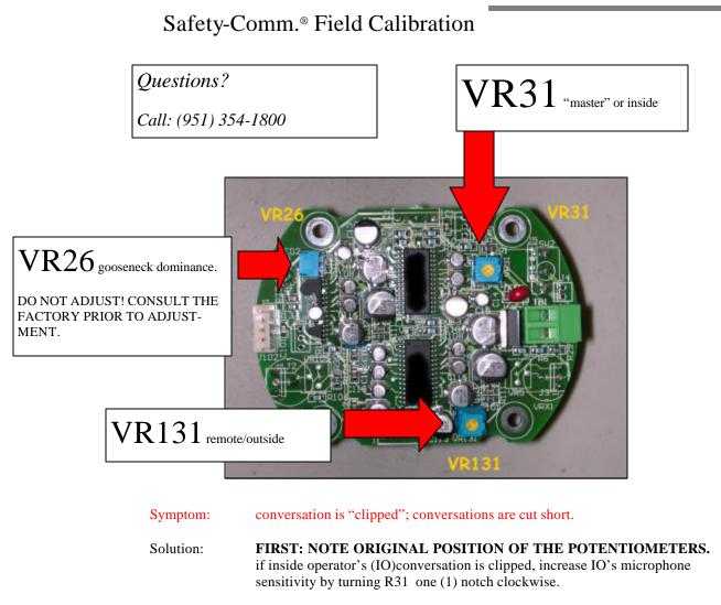
if outside operator's (OO) conversation is clipped, increase OO's microphone sensitivity by turning R131 one (1) notch clockwise.
