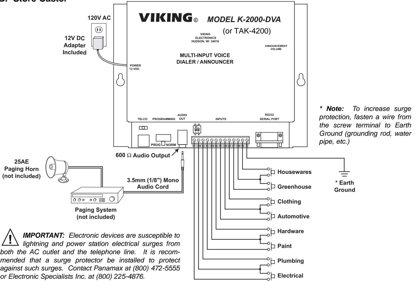
**IMPORTANT:** Electronic devices are susceptible to lightning and power station electrical surges from both the AC outlet and the telephone line. It is recommended that a surge protector be installed to protect against such surges. Contact Panamax at (800) 472-5555 or Electronic Specialists Inc. at (800) 225-4876.
